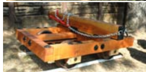
Logging disconnect truck for 24 inch gauge track. This was hand made by Curtis Bonville.
