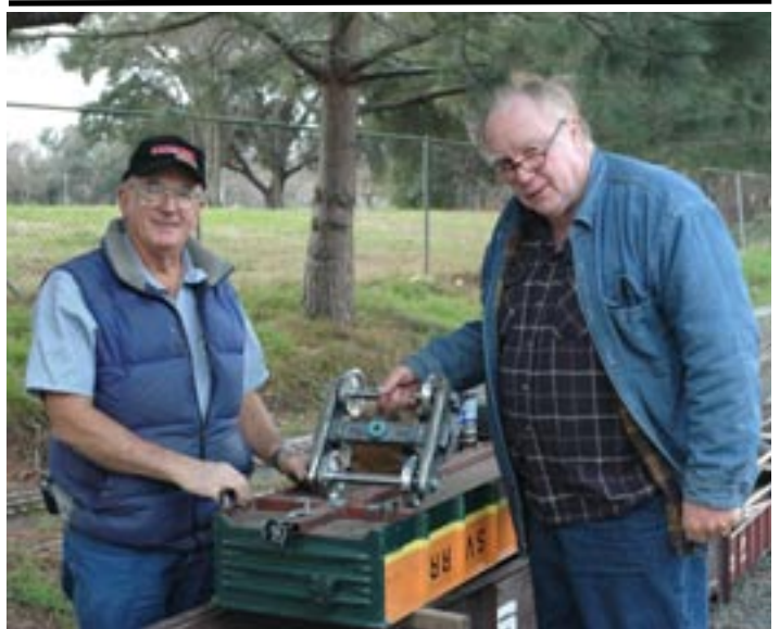
Starting the year working on a SVLS Gondola is Pete Arney and Red Hadler replacing the trucks.
