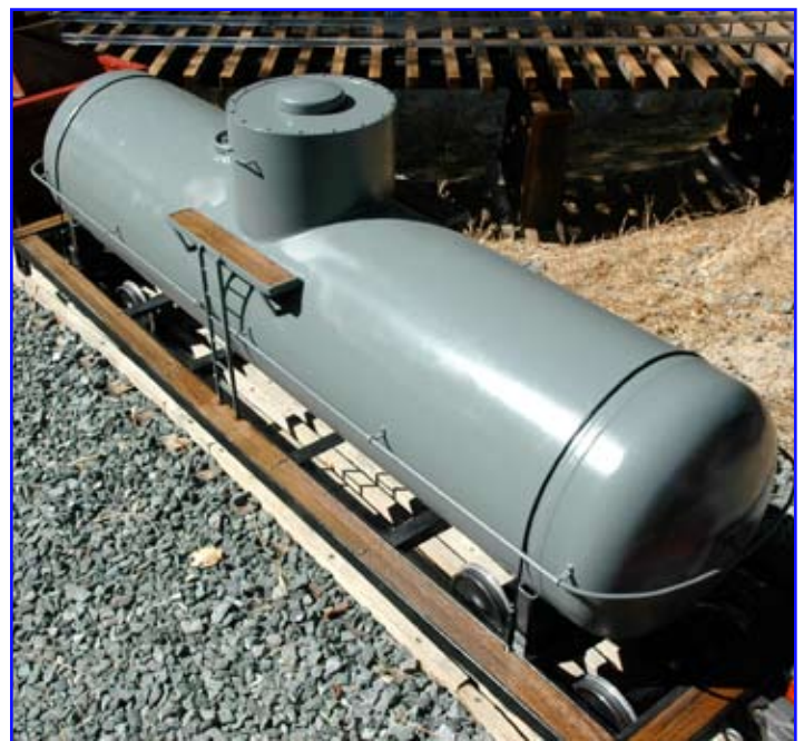
The finished Tank Car is a 5 foot car with a 12" dia. by 54" tank. The walkways are made of oak boards.
