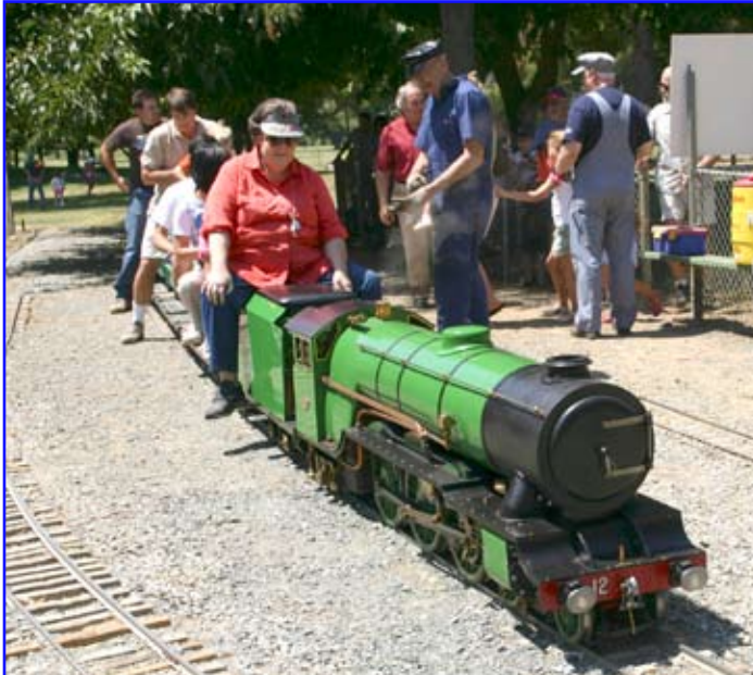
Johns Loco is a 1/2 scale model of the loco on the 15" gauge Romney, Hythe & Dymchurch Railway in the UK.
