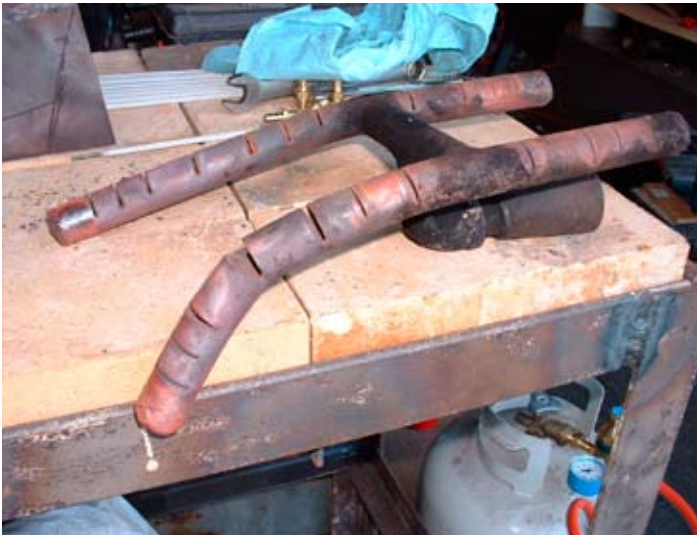
This was the burner being used by our Steamer. As you can see it has warped a new shape.
