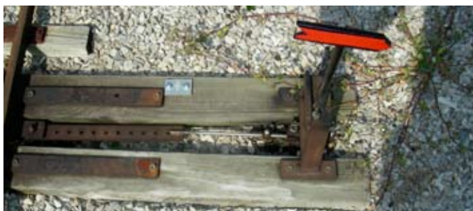
Yard switch indicator, also they have just numbered their switches (small tag in photo)
