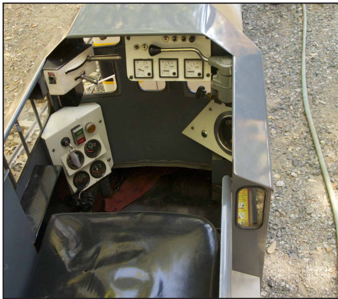
Above picture is the cab of the electric "Vine" engine which shown below uses a gas engine to drive a DC generator which then powers the electric motors in the trucks
