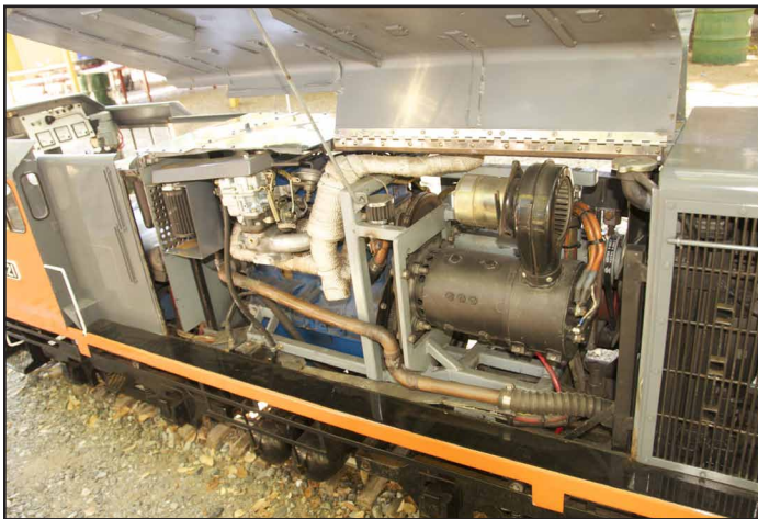
Above picture is the cab of the electric "Vine" engine which shown below uses a gas engine to drive a DC generator which then powers the electric motors in the trucks
