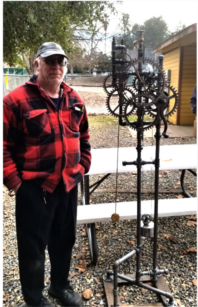
John Bailie shows his home made clock, he designed a unique gear set. Clock will run 36 hours per wind. Thanks for sharing John.
